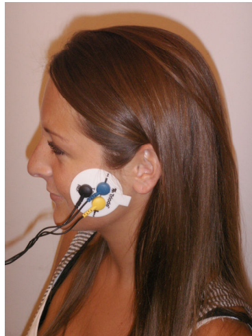
Figure 1: Proper electrode placement of single channel MyoTrac™ EMG device. Ensure the sensor portion of the electrode lies parallel to masseter muscle fibers.
